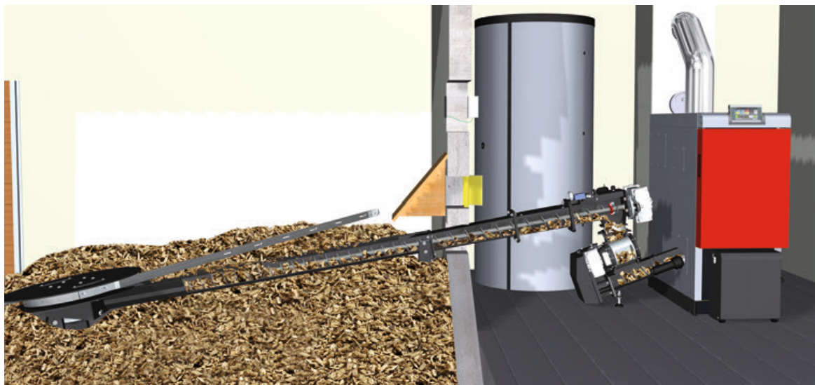
Fig. 42: An automatically fed wood chip heating system with spring core space discharge and screw conveyor for transporting the fuel
