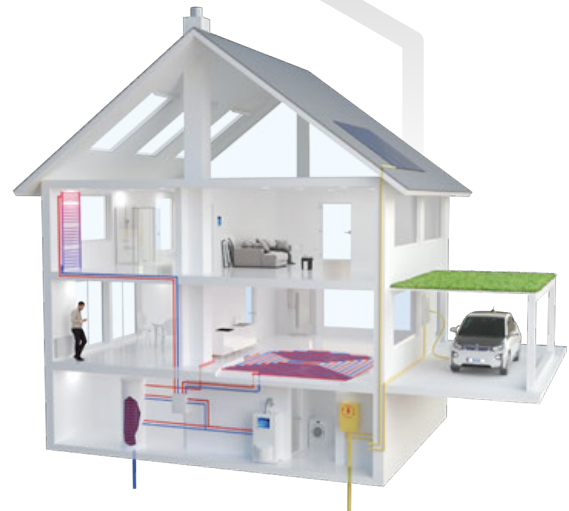
Renovation variant – gas/oil condensing technology
