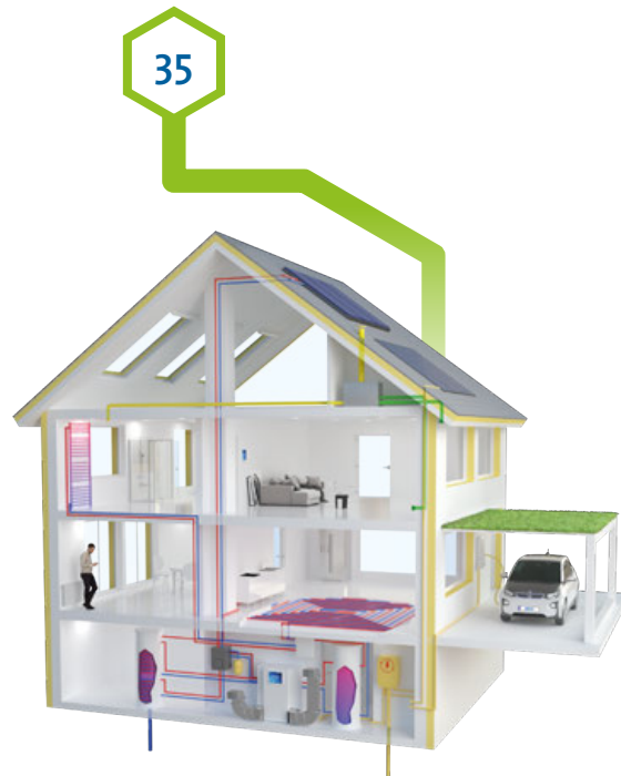
Renovation variant – Air-water heat pump with solar thermal energy, controlled residential ventilation and renovation of the building shell
