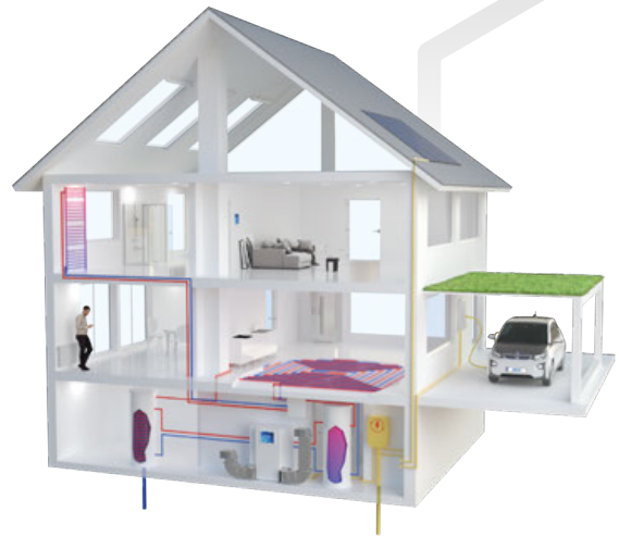
Renovation variant – Air-water heat pump
