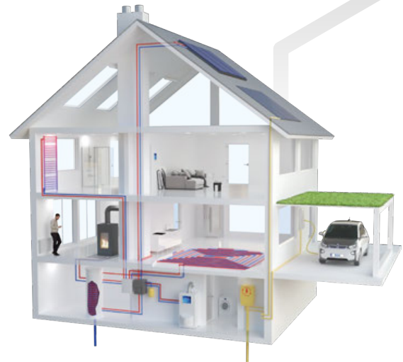
Renovation variant – gas/oil condensing technology with solar thermal energy and wood burning stove/pellet furnace with collection basin
